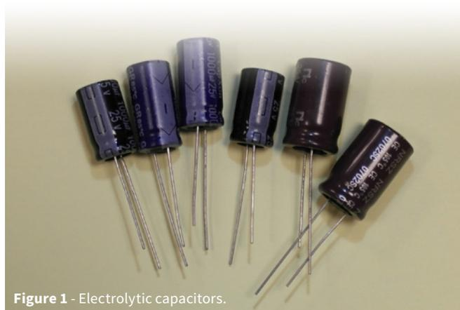
Figure 1 - Electrolytic capacitors.
