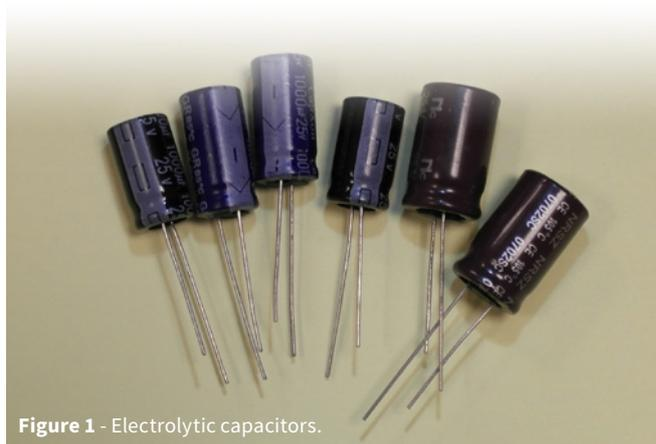
Figure 1 - Electrolytic capacitors.
