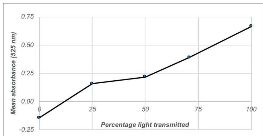
**Figure 3** - Effect of light intensity on the absorbance (525 nm, mean of 5 measurements) of hydrogencarbonate indicator solution. Samples of knotted wrack were immersed in hydrogencarbonate indicator solution and neutral density filters used to reduce the intensity of light incident on the sample. Further experimental details are in the text and the legend to Table 1.
