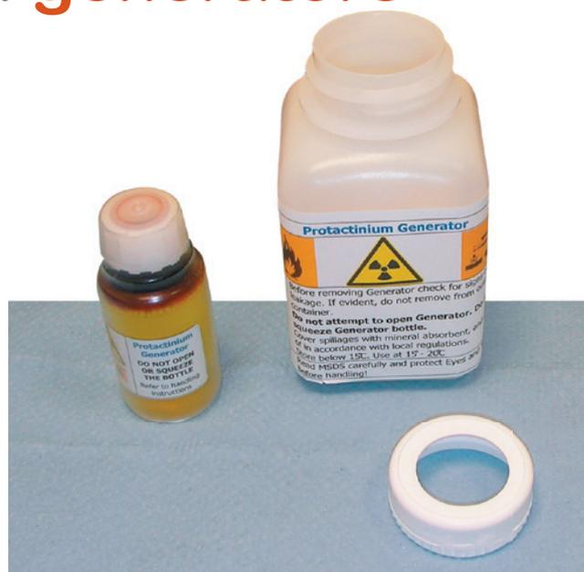
Figure 1 - Protactinium generator.
