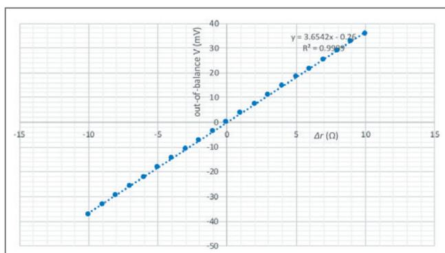
Figure 4 - Out-of-balance  $V$  versus  $\Delta r$ .
