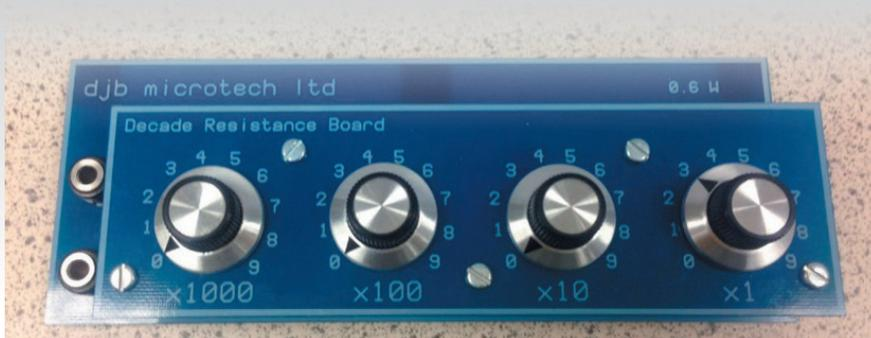
Figure 3 - calibrated variable resistor.
