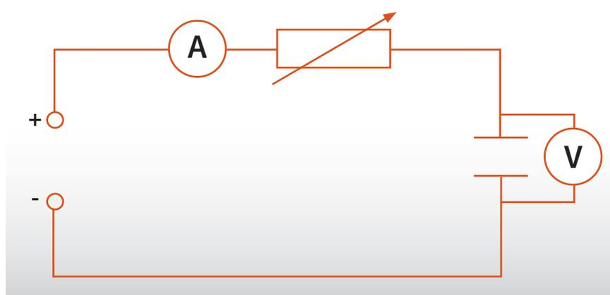
Figure 1 - Capacitor charging circuit.
