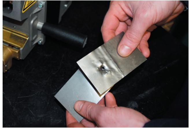
Figure 10 - Testing weld quality.
