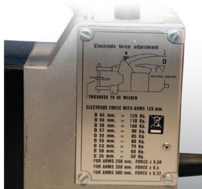
Figure 3 - Weld pressure forces.
