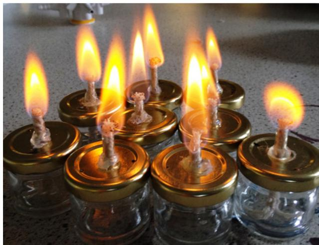
Figure 3 - Homemade spirit burners.
