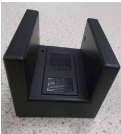
Figure 2 - the BeeSpi V has a pair of light gates.
