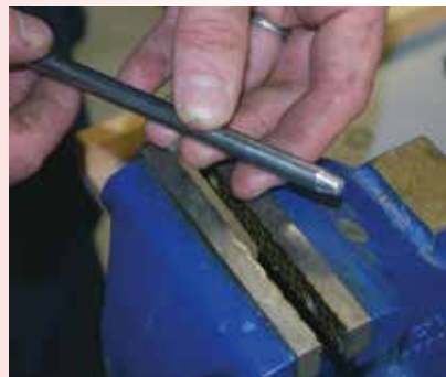
Figure 4 - End of rod tapered to assist start of cut.
