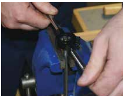
Figure 6 - Die stock is turned clockwise half a revolution.
