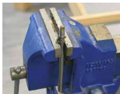
Figure 9 - Completed thread ready for test fit.
