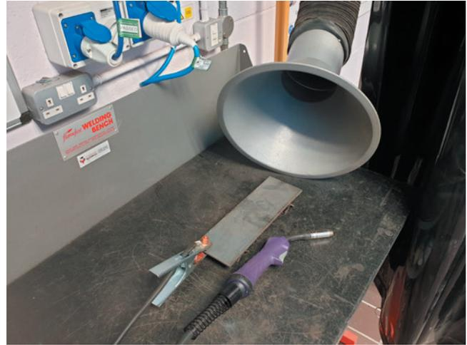
Figure 1 - Welding booth showing movable extraction arm/hood.
