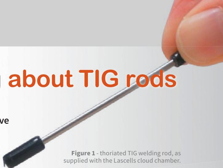
Figure 1 - thoriated TIG welding rod, as supplied with the Lascells cloud chamber.
