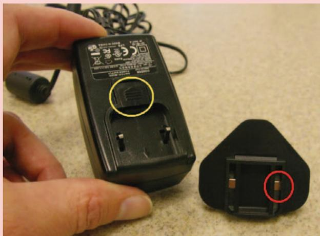
Figure 1 - Plug top with detachable blade.
