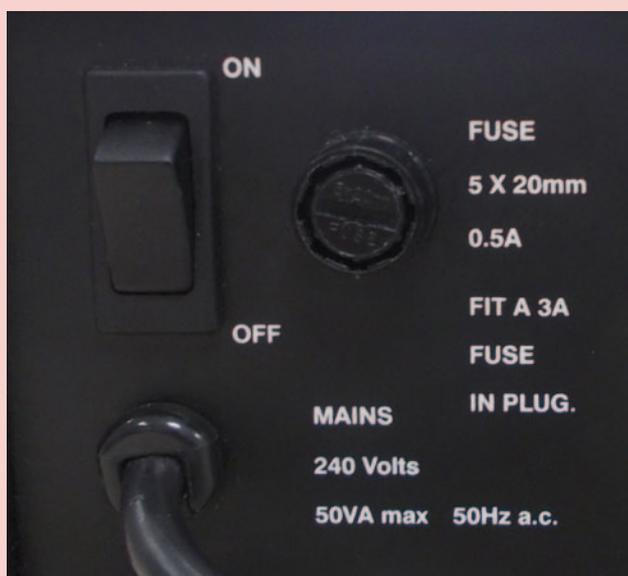
Figure 6 - Rating information on a metal-bodied PSU.
