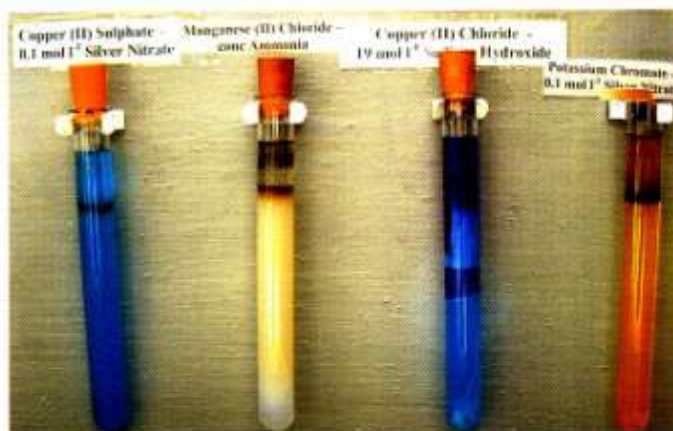
Fig.4 Sodium silicate-based gels after about 8 days
