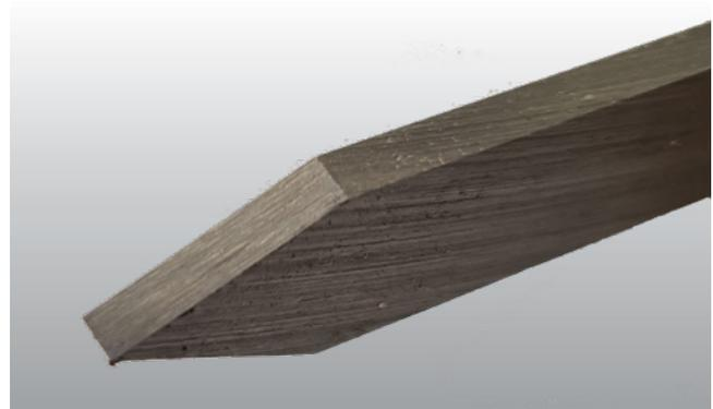
Figure 7 - Parting Chisel.
