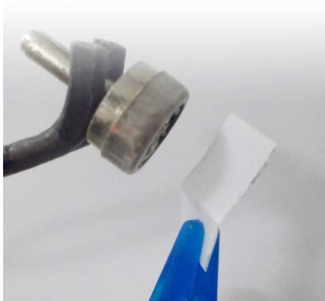
Figure 1 - A source undergoing a leak test.
