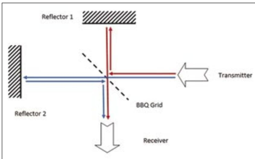
Figure 3 - Beam paths in the interferometer.
