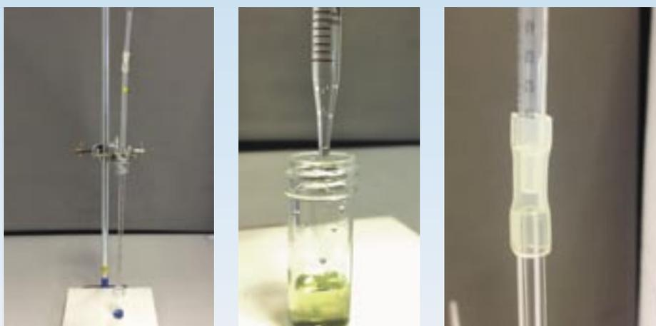
Figure 1 - Microscale titration using a graduated pipette.
