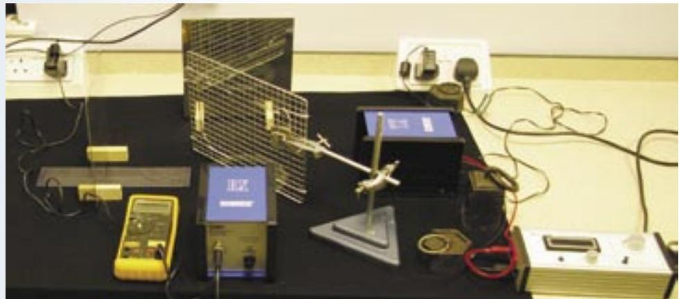
Figure 1 - Microwave Michelson Interferometer.
