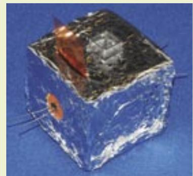
**Figure 10** - Wrap in aluminium foil.
