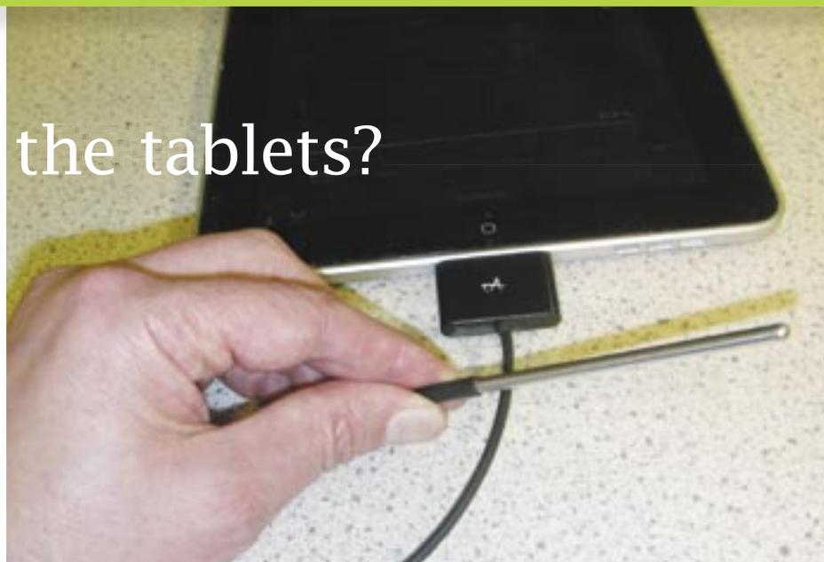
Figure 1 - iPad and iCelsius Pro temperature probe.
