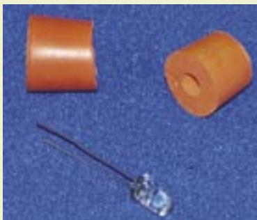
**Figure 3** - Cut bung and LED.
