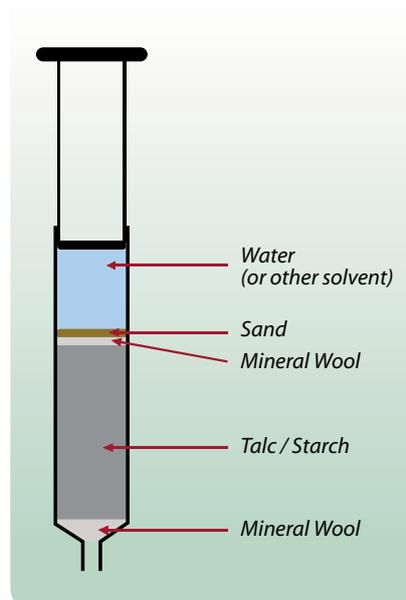
Figure 1 - Setup of syringe.
