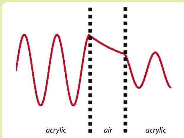
Figure 4 - Transmission across air gap.
