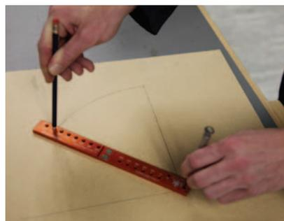
Figure 4 - Diameter/radius marking holes.
