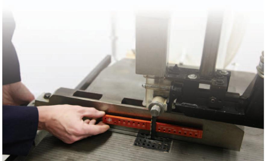
Figure 2 - Central magnets allow the Band Saw Buddy to be attached directly to the blade.
