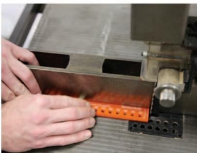
Figure 3 - A 20 mm accurate thickness gauge.
