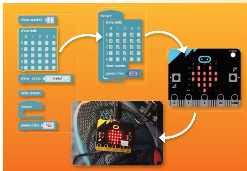
**Figure 1** - Simply click and drag the required commands into a sequence, arrange the timing options of the LED lights as required, then simulate on screen before sending the command to your own micro:bit.
