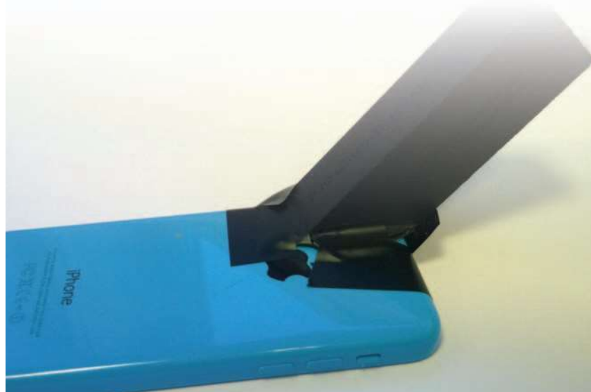
Figure 6 - Spectrometer attached to an iPhone.
