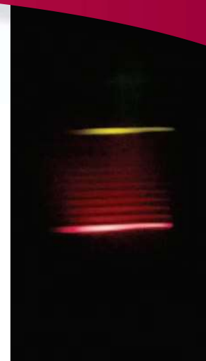
Figure 9 - Spectrum from a strontium flame test.
