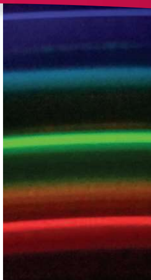
Figure 7 - Spectrum of a compact fluorescent lamp.
