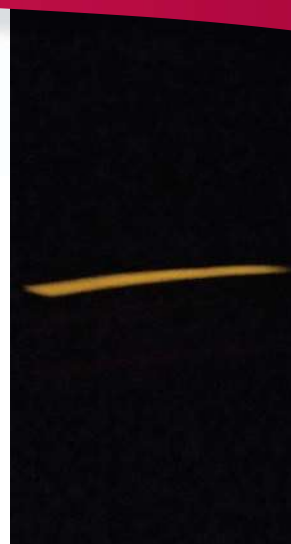
Figure 8 - Spectrum from a sodium flame test.
