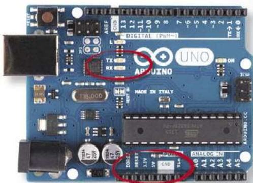
Figure 2 - Power Pins, transmit/receive indicator lights.
