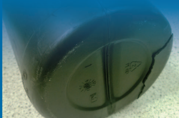
Figure 1 - A nitric acid bottle showing severe cracking.
