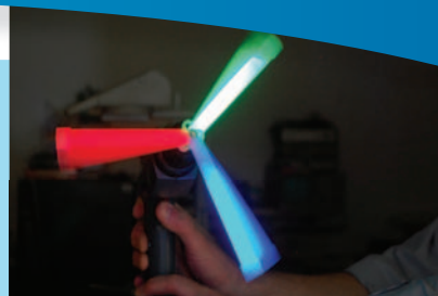
Figure 3 - Lightsticks mounted in the drill assembly.
