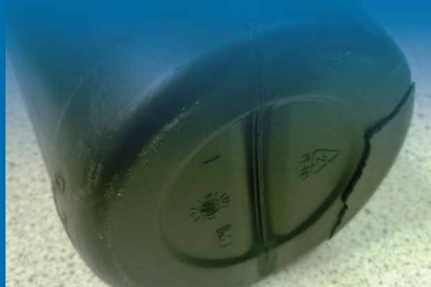
Figure 1 - A nitric acid bottle showing severe cracking.
