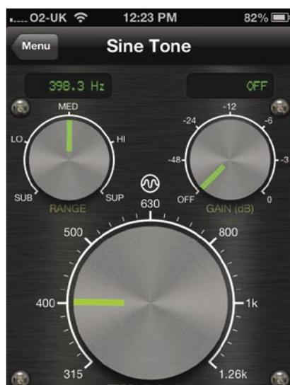
Figure 2 - Smartphone signal generator app.
