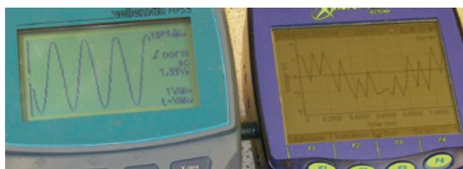
Figure 6 - Velleman and Xplorer at 40 kHz
