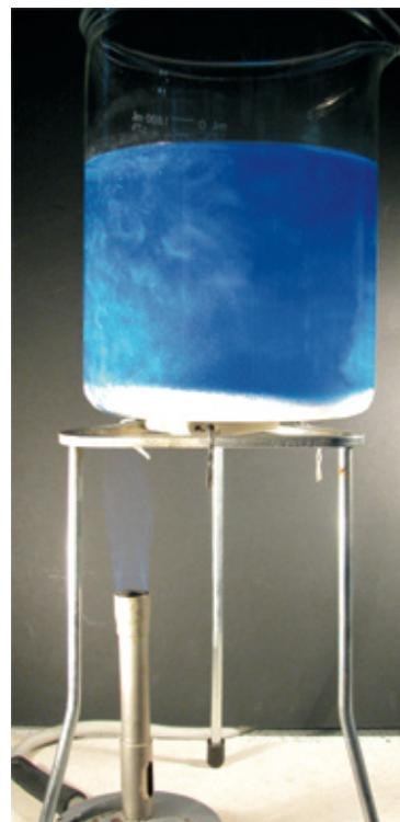
Figure 2 - As liquid is heated the pearlescent particles show convection currents
