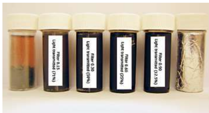
Figure 2: Variation of light intensity using (from left) clear plastic, 71%, 50%, 25%, 12.5% ND filters and aluminium foil
