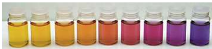
Figure 1: Effects of different concentrations of \text{CO}_2 on the colour of hydrogencarbonate indicator
