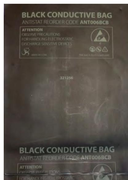
Figure 1 - Black conductive bag made from Velostat.
