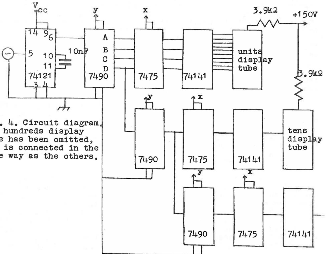
Fig. 4. Circuit diagram. The hundreds display tube has been omitted, but is connected in the same way as the others.
