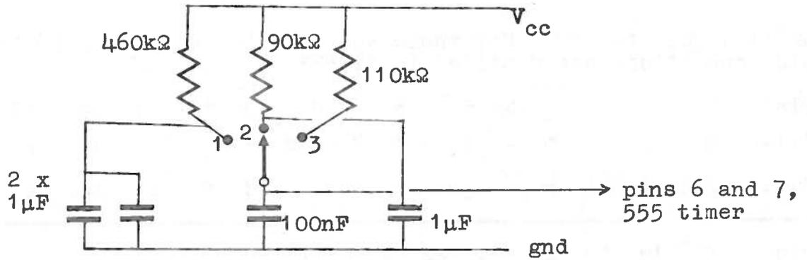
Fig. 5. Frequency range switch. Position 1 = frequency in Hz; position 2, x10; position 3, x100. Resistance values are approximate, and must be adjusted to give 1 s, 100 ms, and 10 ms pulse lengths.
