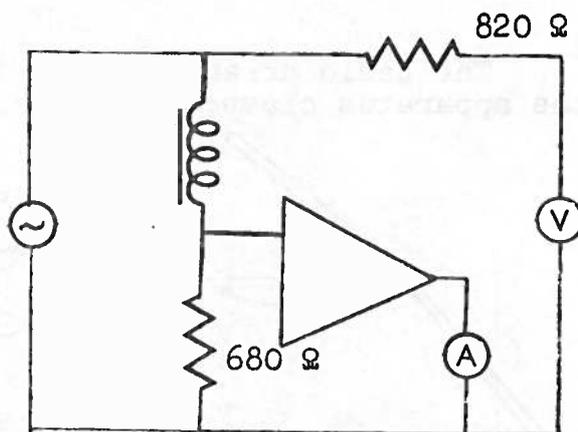
Circuits for H320/3 and H3020/3. Chart speed 5 or 10 mm/s. V and i are recorded on different channels of the recorder.
