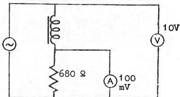
Circuits for CR503. Chart speed 10 mm/s. 10 V and 100 mV are the respective sensitivity ranges for V and i.
