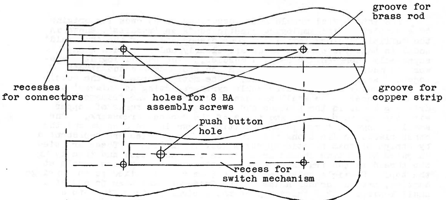
Fig. 1. Plan. Inside view of both halves.
