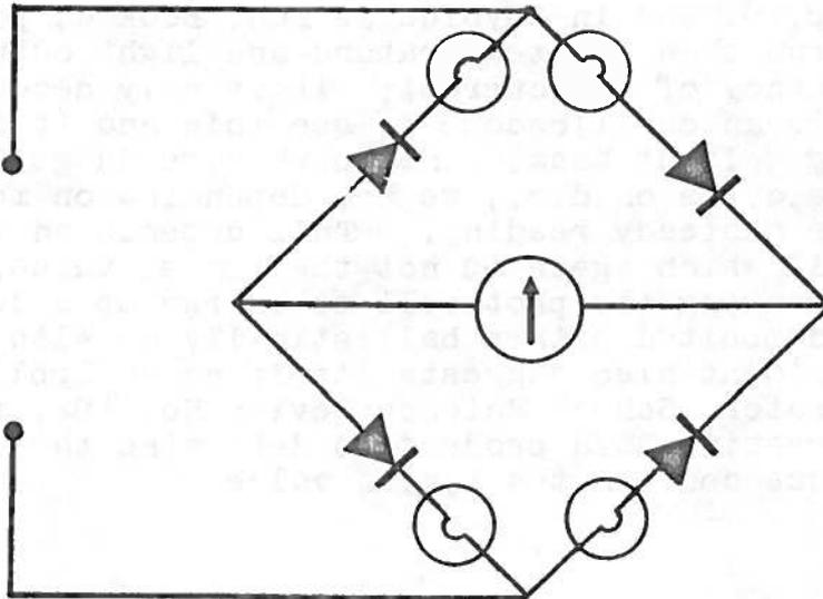
A visitor to our display laboratory has suggested that the functions of lamp as indicator and diode as rectifier can be neatly combined in the one component, viz. the light emitting diode. Suitable l.e.d.s are available at 32p from R.S. Components and some may wish to experiment with this version of the apparatus.
