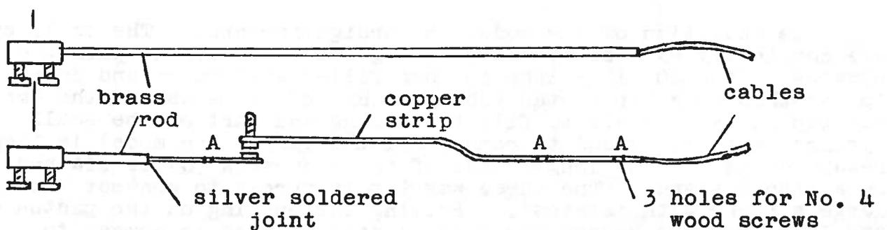
Fig. 2. Elevation. Connectors and switch mechanism.
