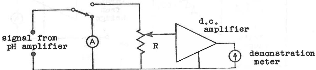
A is the read-out ammeter in the instrument; the switch and all components to the right have to be applied externally.
