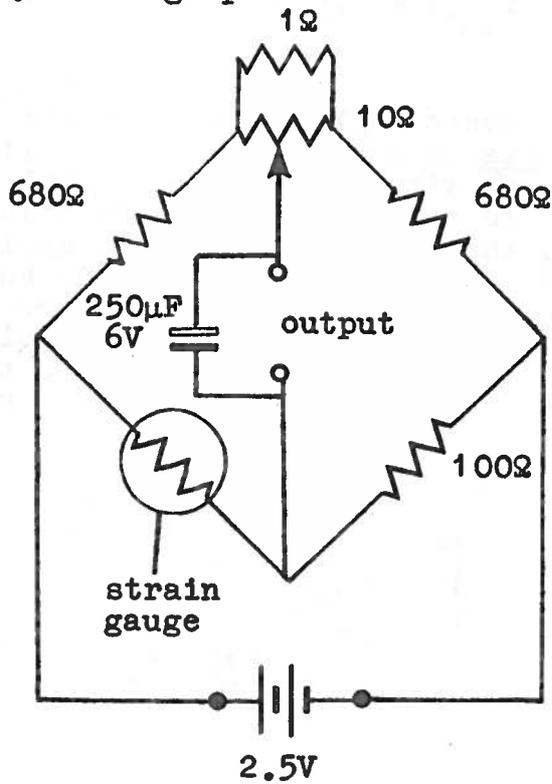
Fig. 3. Bridge circuit
