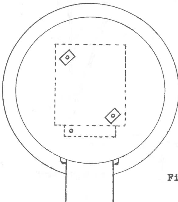
Fig. 3. Rear view of flower pot showing position of adjusting screws.
