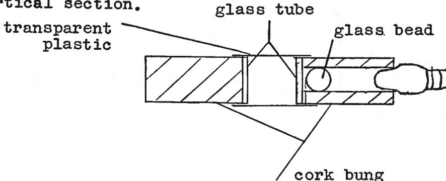
In Bulletin 59 we showed how leads to 4mm plugs could be reinforced by passing them through a hole in the plug so that when pulled the connection would not be stripped from the socket. In the Hirschmann type neoprene plug we brought the lead out through a hole in the side of the plug. A note from Wick High School shows how they have modified the design to allow the wire to leave the plug in the normal way. The sketch below should be self-explanatory.
