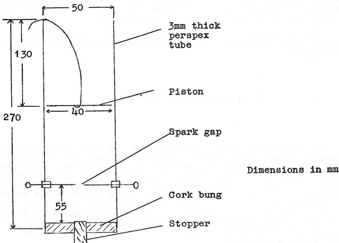
Perspex tube, available from Peter Plastics is convenient for showing the explosions, but the tube could be opaque and of metal; even a convenient size of tin can would do provided there were
