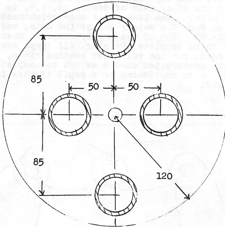
Fig. 2. Plan view of turntable, showing location of ring magnets. Dimensions in mm.
