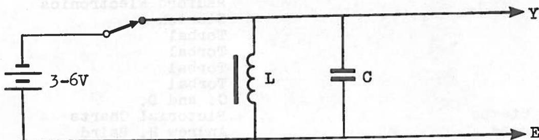
L is the 250 turn section of Unilab LB-3 coil, with a single C core inserted; C is a  $4\mu\text{F}$  paper capacitor and the switch is made up by inserting a piece of copper foil in place of the normal tape in a ticker timer. This gives a recurrent switching action at 50 Hz./
