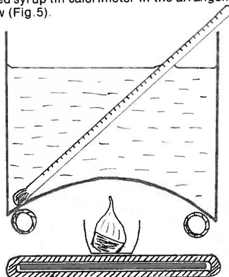
↑ clamped syrup tin lid covered in kaowool to reduce heat loss
