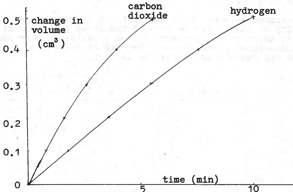
For a pressure difference of 25 mm mercury at  $18^\circ\text{C}$ , the initial rates of flow through balloon rubber stretched to approximately the same tension as that of a three quarters inflated balloon were:
