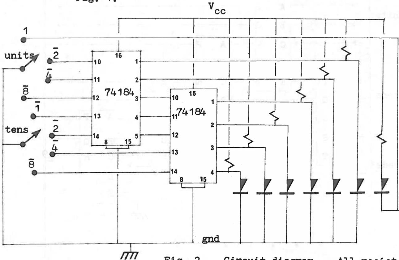
Fig. 2. Circuit diagram. All resistors are 1 k $\Omega$ .
