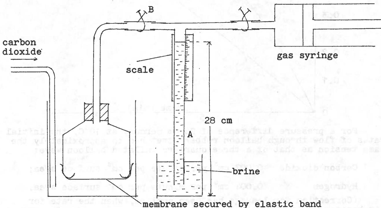
An old BDH concentrated volumetric solution container had a hole cut in its base and the rounded rims left to provide strength. The dimensions of the vertical tube A had to be a compromise. A fine tube would enable more accurate readings of volume to be made, but would suffer from the disadvantages of a large change in pressure as the level fell and from capillarity effects. Standard 6mm outer diameter soda tubing was used.
