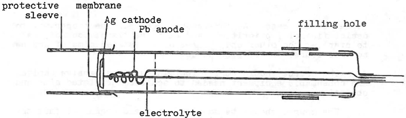
Fig. 1. Galvanic Oxygen Electrode. Note that the normal operating position is vertical.
