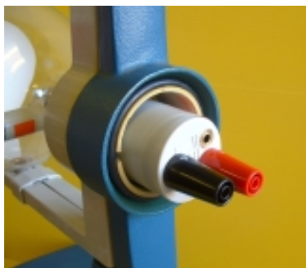
Figure 7 Teltron tube rear sockets adapted for shrouded connectors. In this example, because of insufficient clearance, only 2 sockets can be protected. The red adaptor should be repositioned according to needs.
