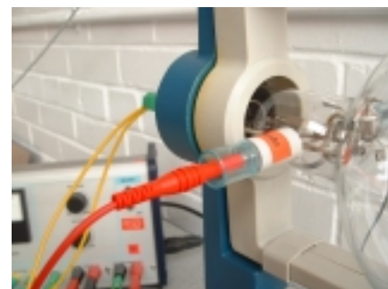
Figure 6 A Teltron electrode protected with its shroud, with a connecting lead through an in-line, 4 mm, free-socket outlet.
