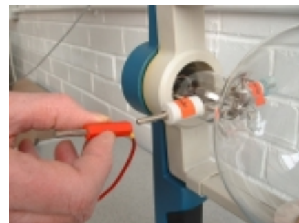
Figure 5 Presenting a stackable, unshrouded, 4 mm plug to an unshrouded electrode on a Teltron tube.
