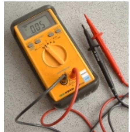
Figure 8 Electrician's digital meter, to show its minimalist features.
