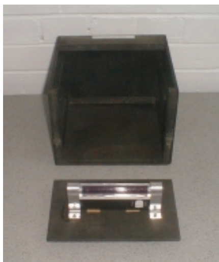
Figure 1 Lightbox interior with front panel removed and lid upturned showing Maplin lamp secured with aluminium brackets.
