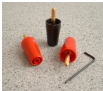
Figure 3 4 mm shrouded connectors. The Allen key is used to turn a screw in the base of the socket, which tightens the fitment.
