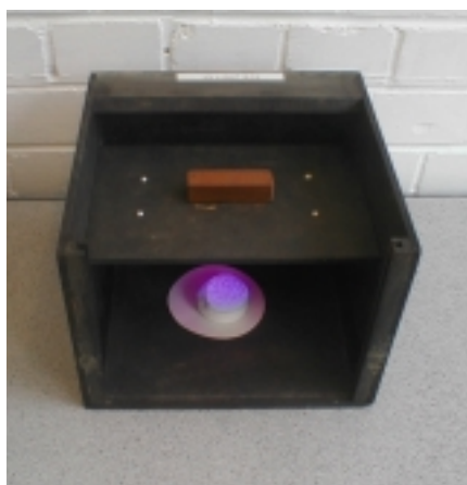
Figure 2 Front panel removed showing a fluorescing specimen (washing powder tablet).
