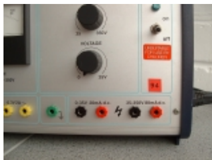
Figure 1 An example of an HT power supply with unshrouded 4 mm socket outlets.
