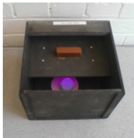
Figure 4 The proper viewing position showing the specimen through the gap between the top and front panels.
