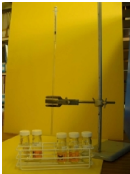
Figure 3 Apparatus set up ready to draw in or expel liquid reagents.
