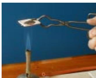
**Figure 2** Metal oxide and carbon being heated on a square of Superwool.
