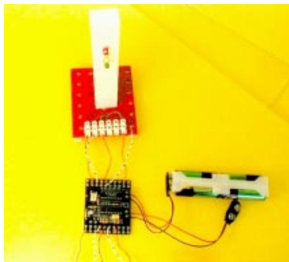
**Figure 2** Fitment of bulbs and holders in model traffic lights.
