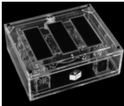
**Figure 1** The Perspex case of the Solar Science Set with its 3 solar panels on the lid and showing 4 output devices down the left hand side.
