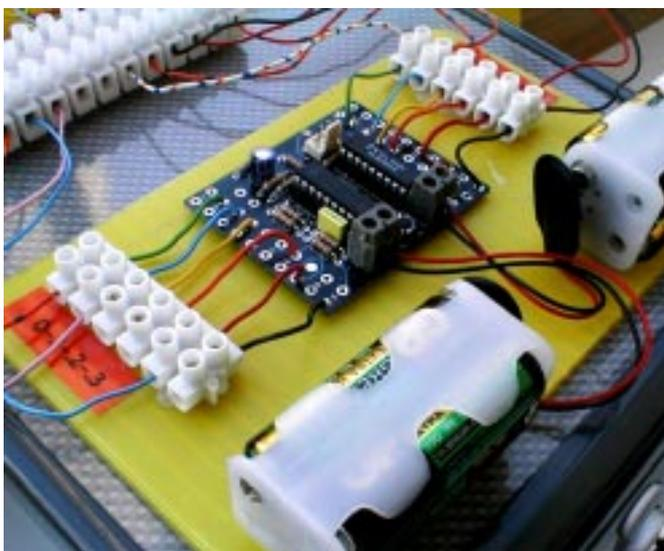
Figure 6 Close-up view of PIC microcontroller on top panel of toy washine machine.
