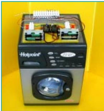
Figure 5 Hotpoint washing machine, toy from Casdon, with PIC controller on top panel.
