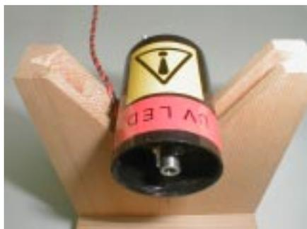
Figure 1 370 nm UV LED in its film canister housing.
