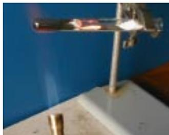
**Figure 1** Potassium permanganate being heated to drive off oxygen; iron is reacting on the other side of a plug of Superwool.
