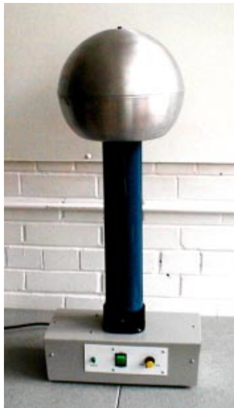
Figure 2 The STE Van de Graaff generator (product code 10178) (dealers include Anderson Scientific (10178), Griffin (XJE-350-V) and Scientific & Chemical (XES 030 010)).
