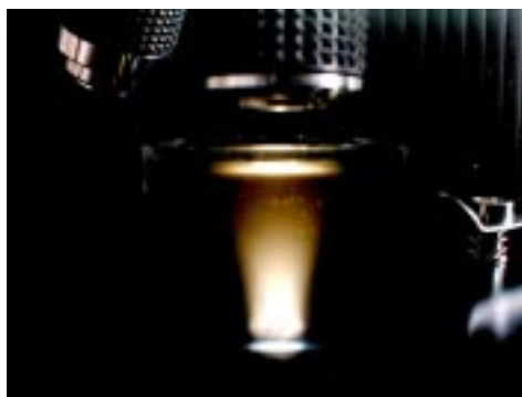
Figure 2 Correctly illuminated specimen and objective with the condenser focussed and the iris diaphragm properly adjusted. This should assist in achieving optimum resolution with good contrast and adequate control of glare.
