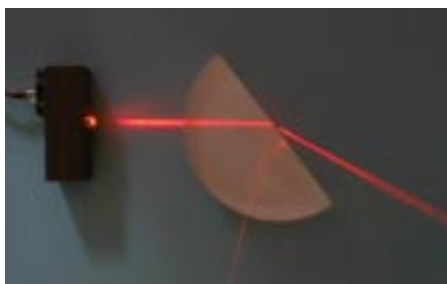
Figure 3 The LM-04 line generator used as a ray source. Shows refraction at a semi-circular block.
