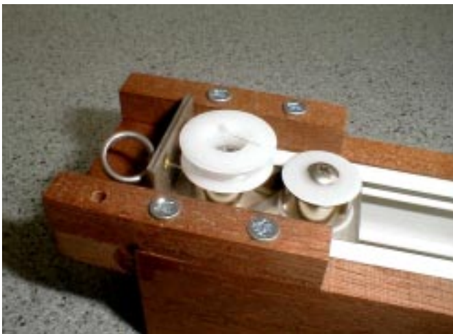
Figure 1 Photograph of a Constant Force Spring (McMaster Carr product 61115A1) in a home-made mount.
