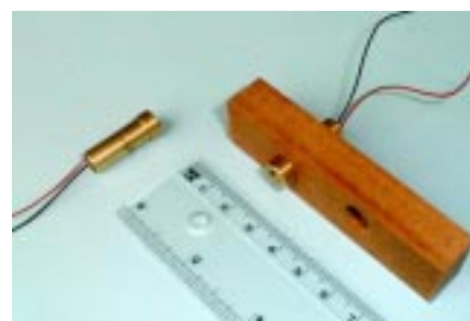
Figure 2 Two LM-04 line generators, the one on the right being fitted to a hardwood block, which serves as a clamp.
