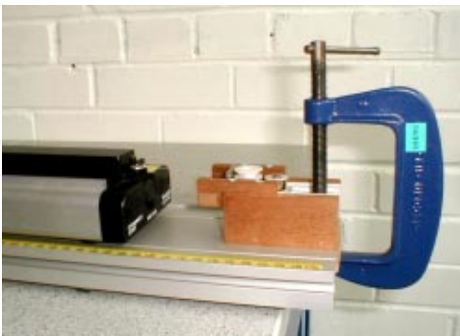
Figure 2 Photograph of a PASCO Dynamics Cart attached to a Constant Force Spring.
