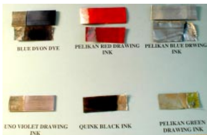
Figure 2 Examples of dyed anodised aluminium strips.
