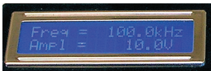
Figure 5b - Digital display with frequency & output voltage.
