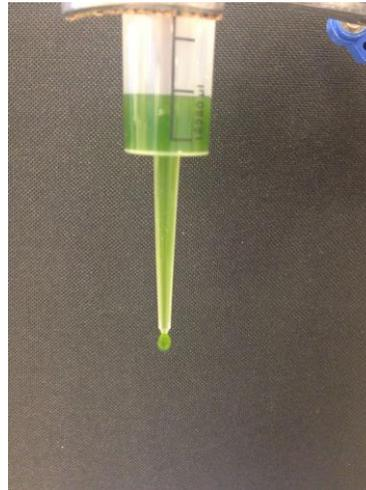
6. As the algae/alginate mixture flows into the CaCl<sub>2</sub> solution you should see that small spherical beads of immobilised algae are formed.
