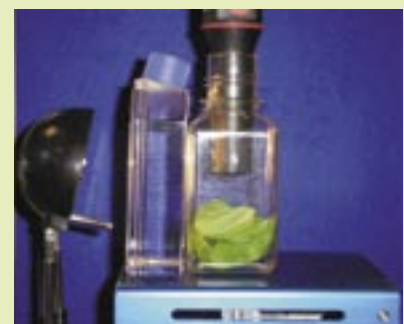
Figure 2 - Experimental set-up for measuring respiration and photosynthesis rates in plants.
