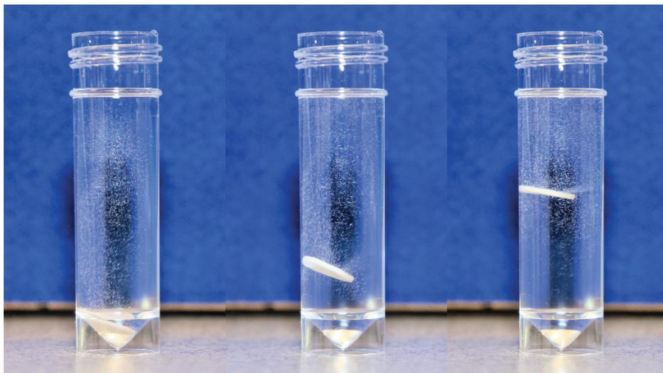
**Figure 1** - A single drop of a 1% suspension of yeast has been added to a filter disc and then placed in a 1% solution of hydrogen peroxide. Photographs were taken at (approximately) 3 s (A), 8 s (B) and 13 s (C).
