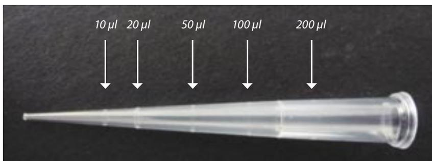
Figure 3 - Syringe tip showing graduation marks.
